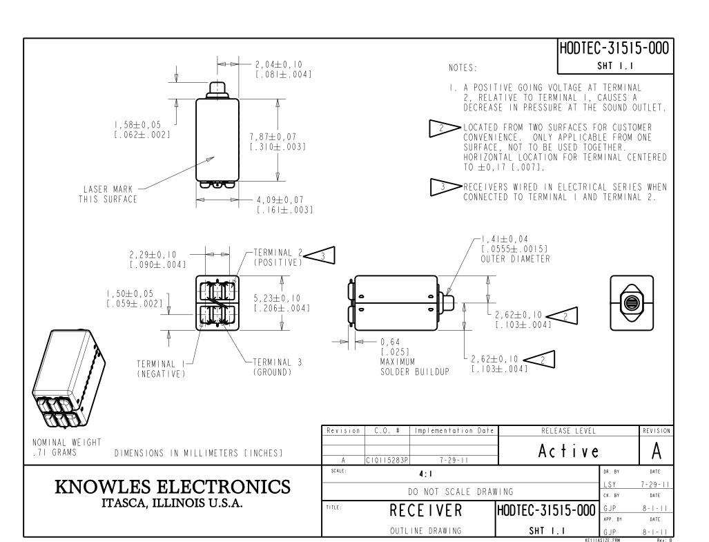
THE HODTEC-31515-000 IS A PAIR OF BALANCED ARMATURE RECEIVERS INTENDED FOR USE IN HIGH POWER HEARING AIDS. IT HAS A MEDIUM DCR TO IMPEDANCE RATIO AND IS A SIMILAR SIZE TO AN EF RECEIVER.
